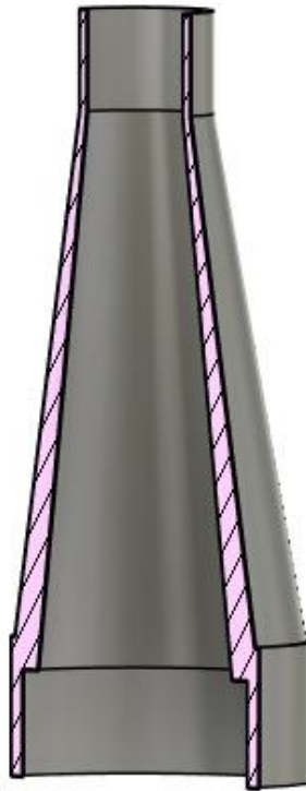
Figure 22: Cross-section of Optical Housing
